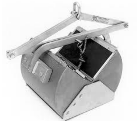
Figure 7. Petite ponar sampler for use in lakes and non-wadeable streams
