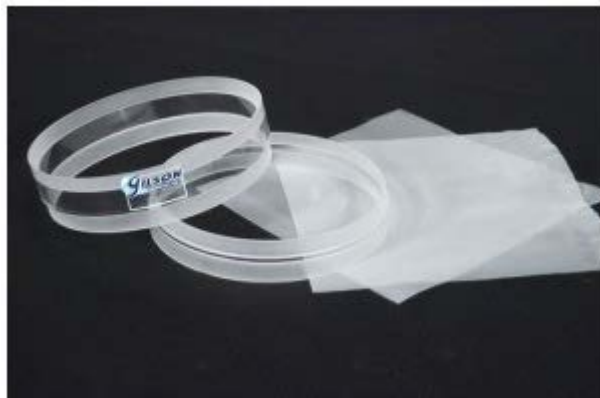
Figure 10. Sieve mesh and sieve frame for sediment sample processing
