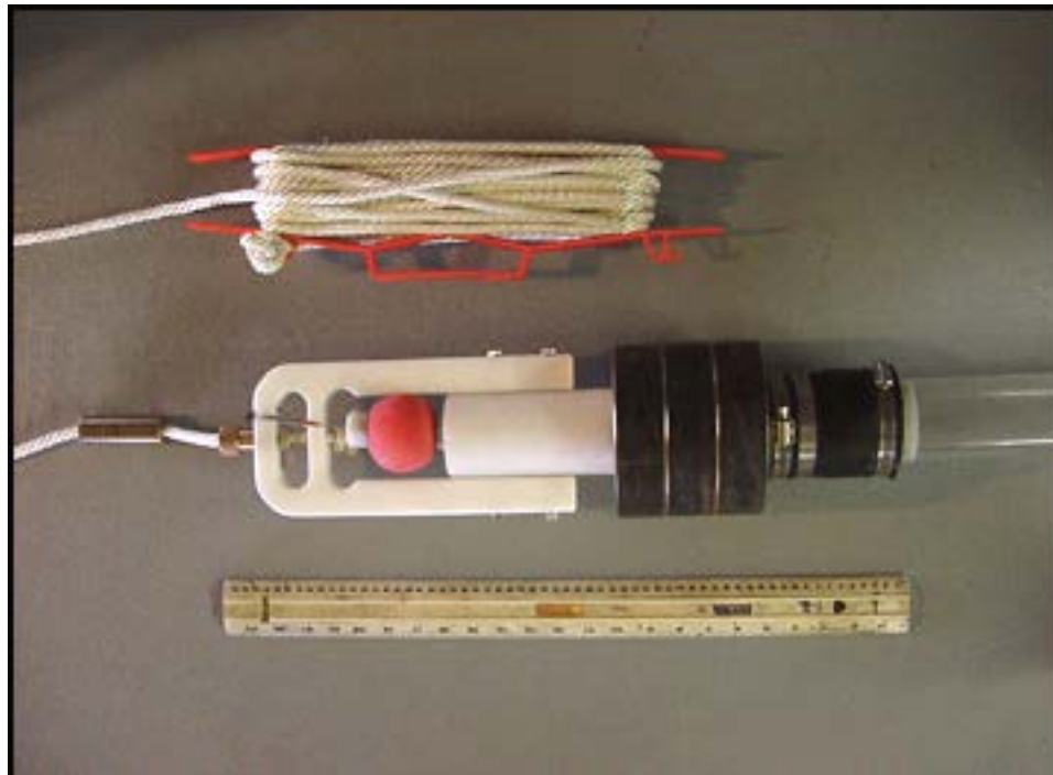
Figure 8. Gravity corer sampler for use in lakes and non-wadeable streams
