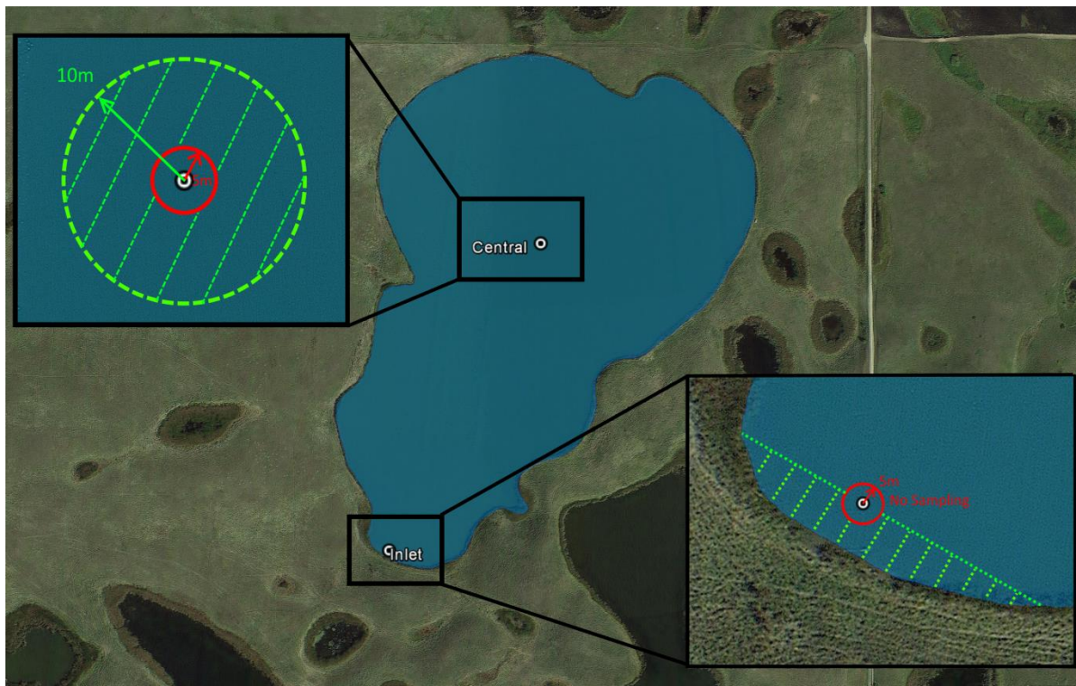
Figure 6. Example lake sediment collection stations with sensor exclusions areas (red) and sampling zones (green).
