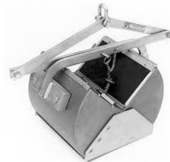
Figure 8. Petite ponar sampler for use in lakes and non-wadeable streams
