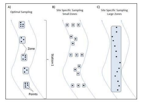
Figure 9. Diagram to exemplify determination of sampling zones in non-wadeable streams based on site differences. A) Ideal sampling set up based on availability of different depositional zones (~1 m<sup>2</sup>); B) in sites with only random small pockets of sediment; and C) in sites where most of the stream bed is characterized by sedimentary or organic substrate.
