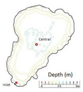
**Figure 3.** Identifying the Station for sediment sampling in lakes. The two sampling Stations (red circles) should denote depositional zones in the center of the lake (deepest section) and in a nearshore depositional environment
