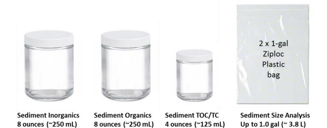
**Figure 4.** Example of clear Boston round glass jars with PTFE lined lid used for collecting sediment for inorganics, organics (PAH/PCB), and TOC/TC analyses. Sediments for grain size samples are collected by filling 2 1-gallon (~3.8L) plastic Ziploc bags about half-full.
