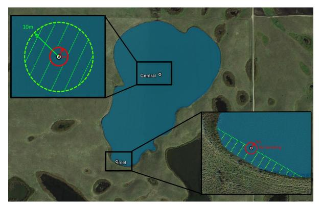
Figure 8. Example lake sediment collection stations with sensor exclusions areas (red) and sampling zones (green).
