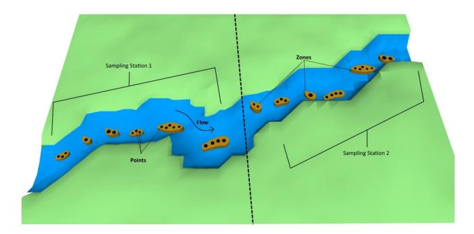
**Figure 1.** Identifying the location for sediment sampling in non-wadeable streams. The two sediment sampling stations should contain depositional zones that represent upstream influences and various flow regimes.
