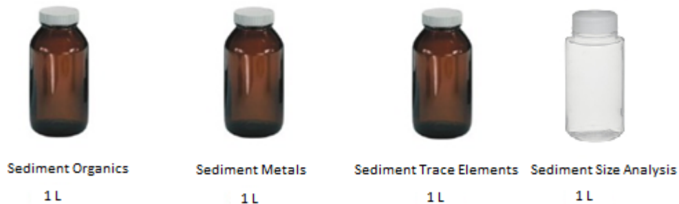
Figure 4. Example of Amber bottles used for collecting organics, metals and trace elements and a Teflon bottle for sediment size samples.
