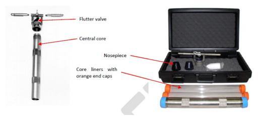
Figure 9 Hand corer for use in wadeable streams with fine sediments
