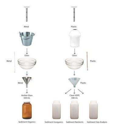
Figure 10 Sediment collection instruments by sample type
