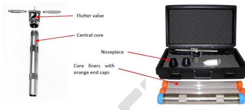
Figure 10. Hand corer for use in wadeable streams with fine sediments
