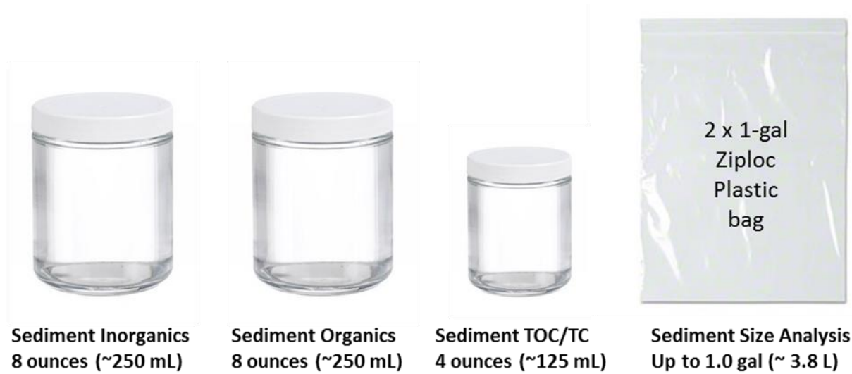
Figure 6. Example of clear Boston round glass jars with PTFE lined lid used for collecting sediment for inorganics, organics (PAH/PCB), and TOC/TC analyses. Sediments for grain size samples are collected by filling 2 1-gallon (~3.8L) plastic Ziploc bags about half-full.
