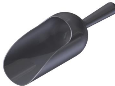
Figure 7. Scoop samplers composed of metal, plastic or glass are used for collecting sediment in wadeable streams
