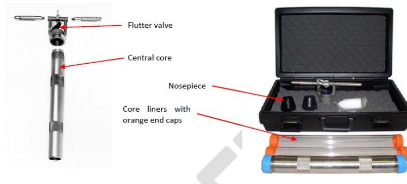
Figure 13. Hand corer for use in wadeable streams with fine sediments
