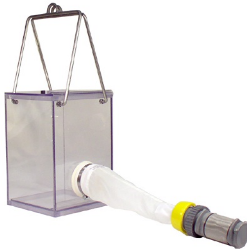
Figure 8. Example of a Schindler-Patalas sampler
