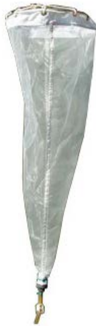
Figure 5. Zooplankton Tow Net
