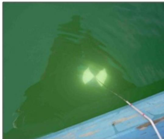
Figure 5. Taking a Secchi Disk measurement on the shaded side of the boat.
