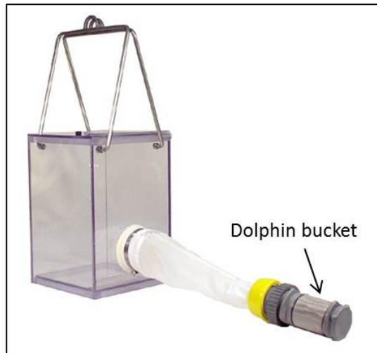
Figure 9. Example of a Schindler-Patalas sampler
