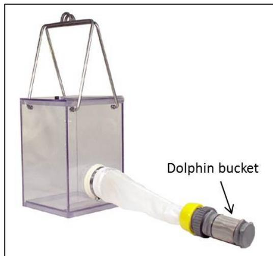
Figure 9. Example of a Schindler-Patalas sampler
