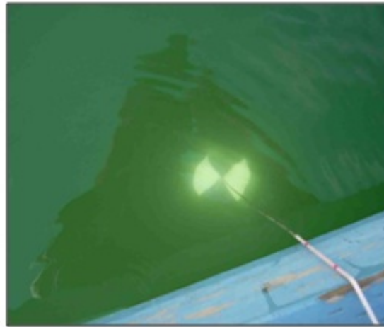
Figure 6. Taking a Secchi Disk measurement on the shaded side of the boat.
