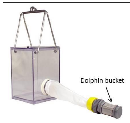
Figure 5. Example of a Schindler-Patalas sampler with Dolphin bucket.
