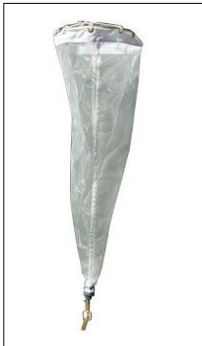
Figure 7. Zooplankton tow net with bottom tubing and clamp.
