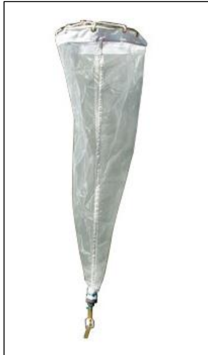
Figure 9. Zooplankton tow net with bottom tubing and clamp.
