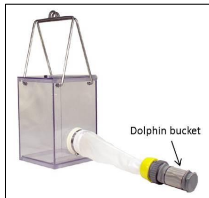
Figure 6. Example of a Schindler-Patalas sampler with Dolphin bucket.
