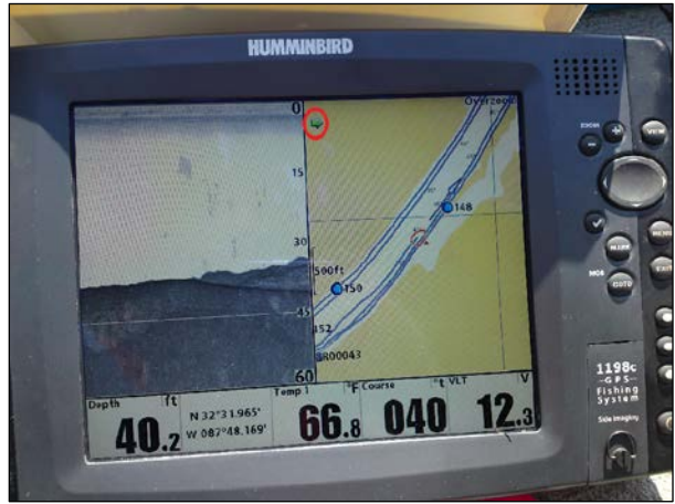
Figure 7. Example of screen with green arrow pointing to the currently “active side” (referenced by the red circle).
