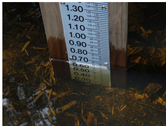
Figure 5. Example of a staff gauge. If conditions are wavy note the mean height.
