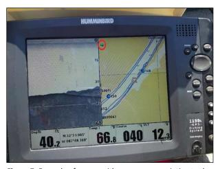
**Figure 7.** Example of screen with green arrow pointing to the currently "active side' (referenced by the red circle)
