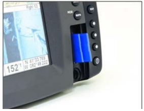
Figure 4. Insertion of SD cards in HumminBird card slot
