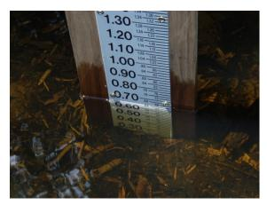
**Figure 5.** Example of a staff gauge. If conditions are wavy note the mean height.
