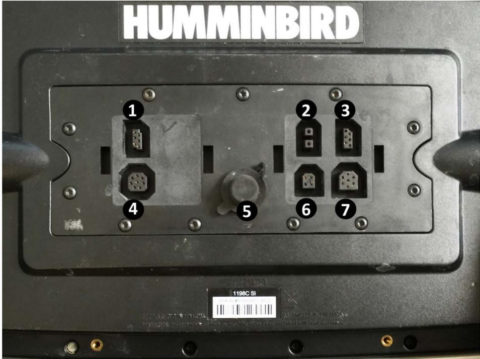
**Figure 4.** Rear view of the HumminBird control panel with connector details. 1) Video-Out (RS-232), 2) Power, 3) GPS/Communications, 4) Video Out, 5) Ethernet, 6) Temperature/speed, and 7) Transducer
