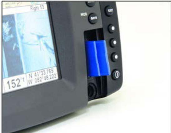
**Figure 5.** Insertion of SD cards in HumminBird card slot
