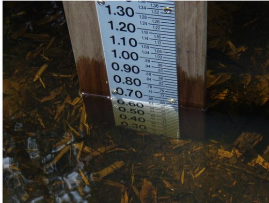
**Figure 6.** Example of a staff gauge. If conditions are wavy note the mean height.
