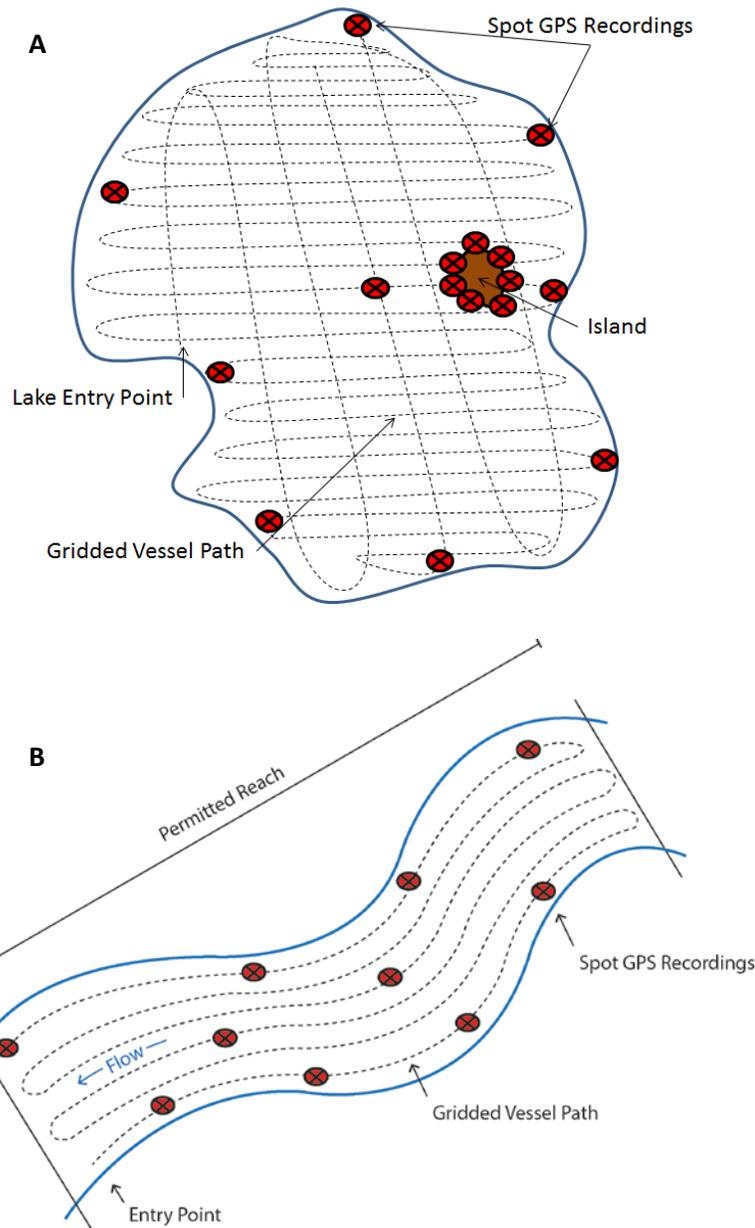
**Figure 9.** Schematic of gridded pattern undertaken in the vessel and approximate locations for (A) lake shoreline and island point GPS measurements as well as (B) non-wadeable stream GPS measurements
