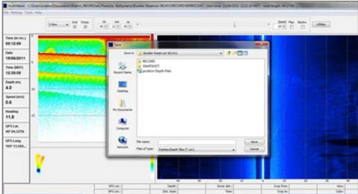
**Figure 13.** Process for exporting the Lat/Long and Depth data in .CSV format for data pre-processing and eventual import into ArcGIS for the bathymetric map data product
