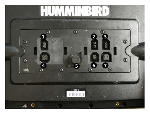
**Figure 4.** Rear view of the HumminBird control panel with connector details. 1) Video-Out (RS-232), 2) Power, 3) GPS/Communications, 4) Video Out, 5) Ethernet, 6) Temperature/speed, and 7) Transducer
