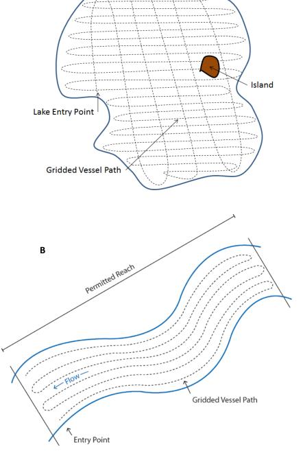
**Figure 1.** Grid pattern used for determining the (A) lake and (B) non-wadeable bathymetry and morphology
