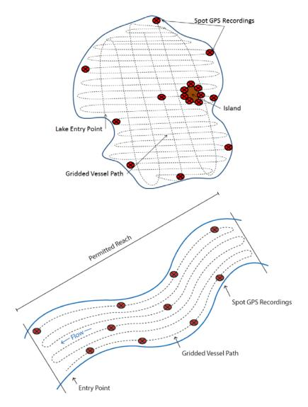
**Step 9** – Take 10 spot measurements around the lake or along the stream reach of GPS coordinates with the handheld GPS and collect and record GPS coordinate of the deepest part of the water body
