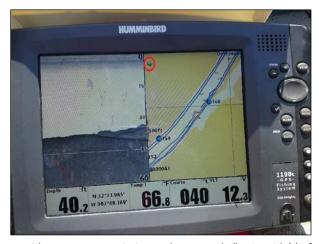
Figure 8. Example of screen with green arrow pointing to the currently "active side" (referenced by the red circle)
