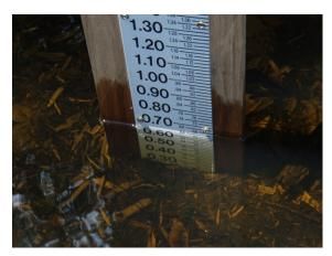
Figure 6. Example of a staff gauge. If conditions are wavy note the mean height.
