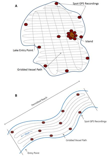
**Figure 9.** Schematic of gridded pattern undertaken in the vessel and approximate locations for (A) lake shoreline and island point GPS measurements as well as (B) non-wadeable stream GPS measurements
