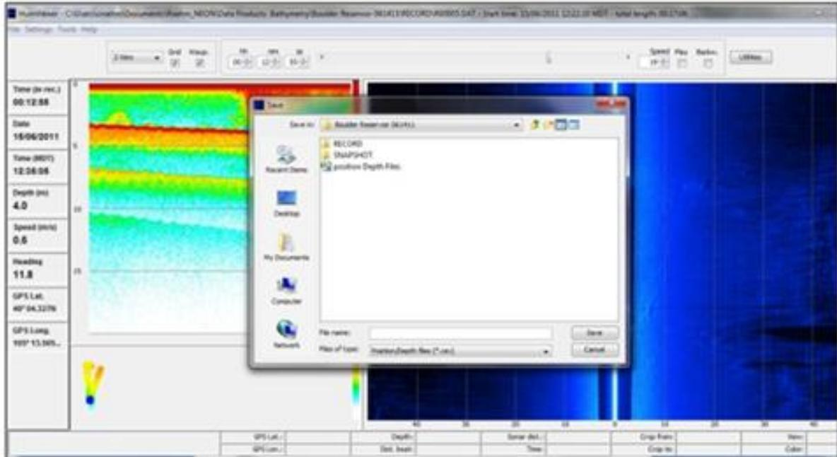
**Figure 14.** Process for exporting the Lat/Long and Depth data in .CSV format for data pre-processing and eventual import into ArcGIS for the bathymetric map data product
