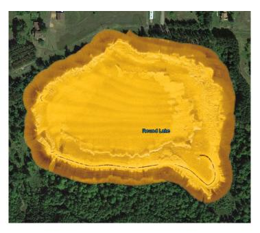
Figure 2. Example of side-scan mosaic master image of a lake bottom.
