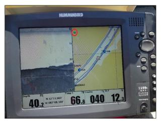
Figure 9. Example of screen with green arrow pointing to the currently "active side' (referenced by the red circle)
