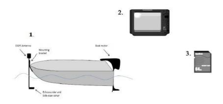
**Figure 3.** Bathymetric mapping system components. 1) Placement of sounder and transducer on the boat; 2) HumminBird main control panel; and 3) SD memory cards
