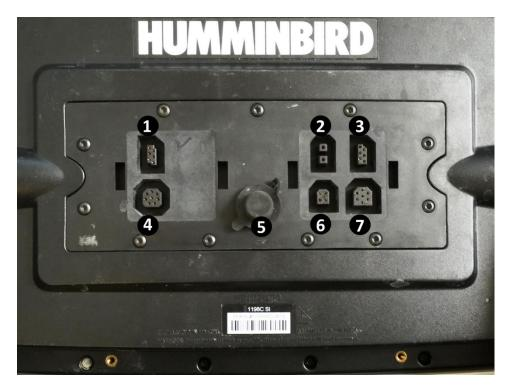
**Figure 5.** Rear view of the HumminBird control panel with connector details. 1) Video-Out (RS-232), 2) Power, 3) GPS/Communications, 4) Video Out, 5) Ethernet, 6) Temperature/speed, and 7) Transducer
