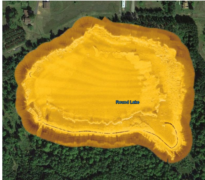
Figure 2. Example of side-scan mosaic master image of a lake bottom.
