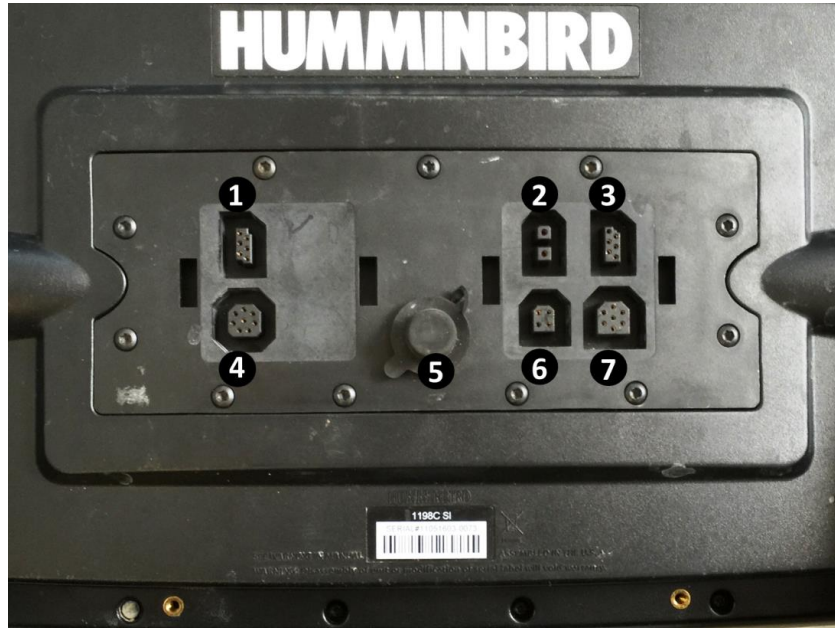
Figure 7. Rear view of the Humminbird control head with connector details. 1) Video-Out (RS-232), 2) Power, 3) GPS/Communications, 4) Video Out, 5) Ethernet, 6) Temperature/speed, and 7) Transducer
