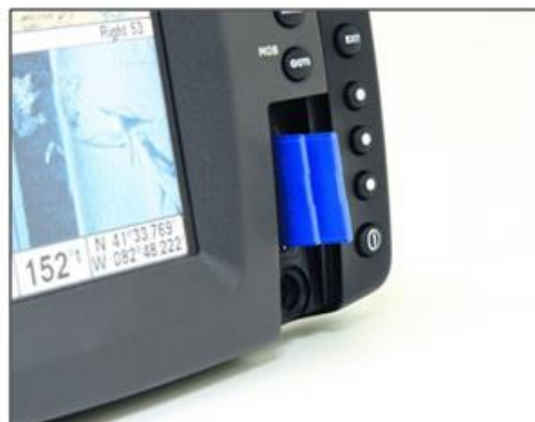
Figure 8. Insertion of SD cards in Humminbird card slot
