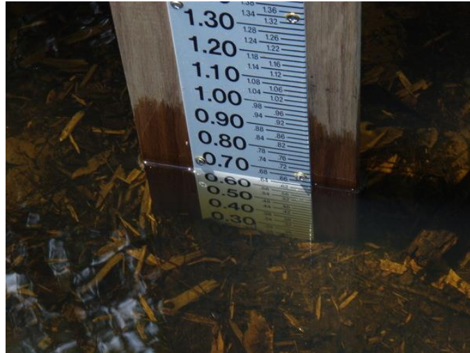
Figure 10. Example of a staff gage. If conditions are wavy note the mean height.
