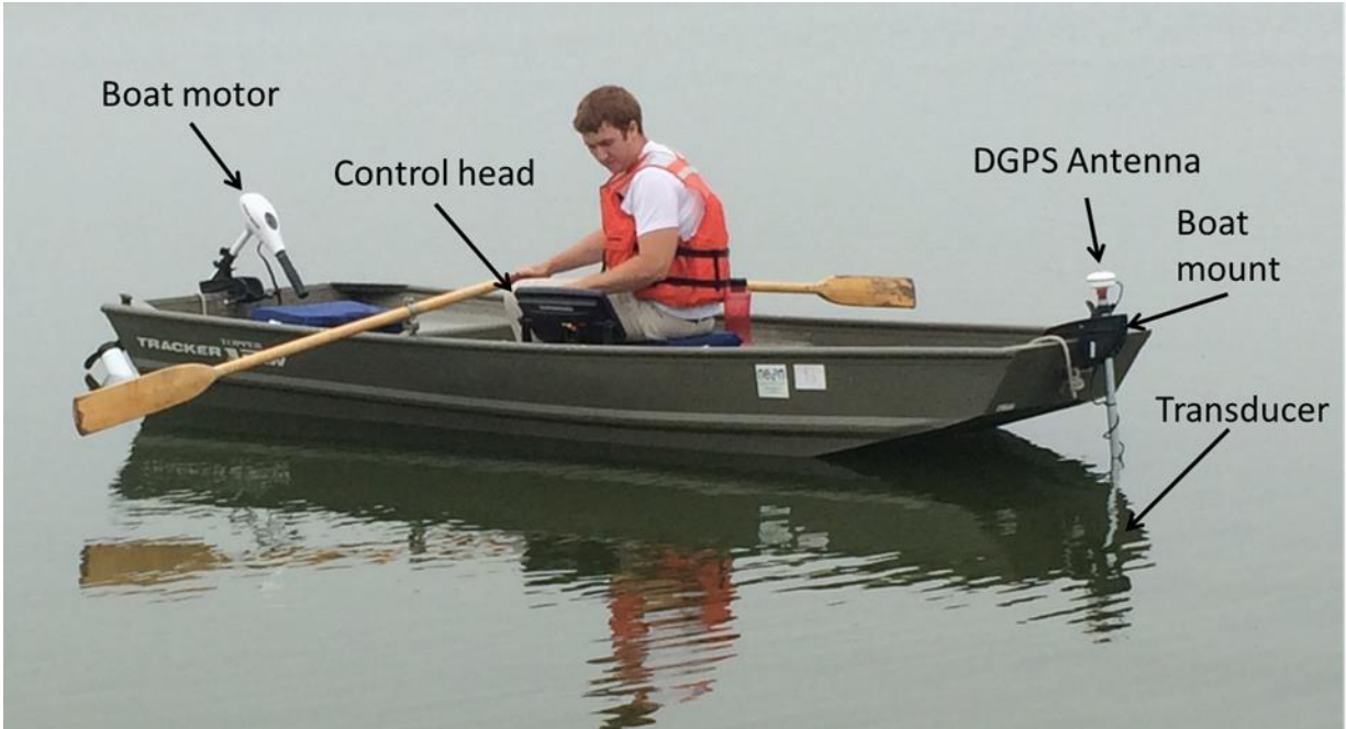
Figure 5. Bathymetric mapping system components.
