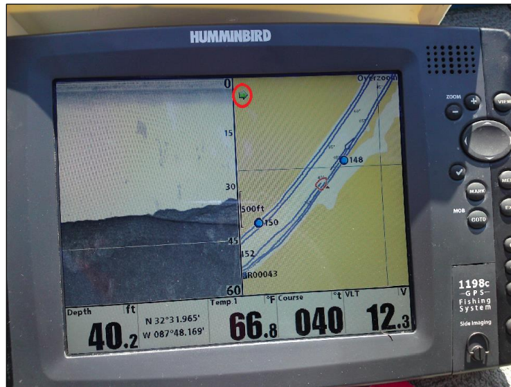
Figure 14. Example of screen with green arrow pointing to the currently “active side’ (referenced by the red circle)
