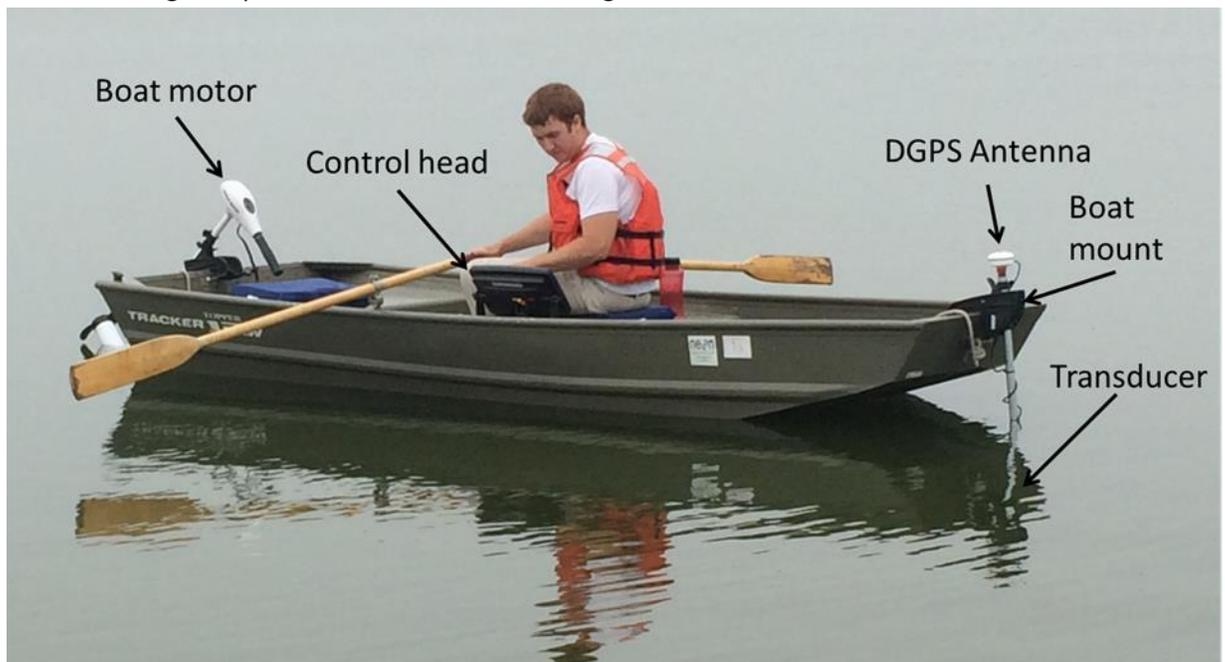
**Figure 5.** Bathymetric mapping system components.
