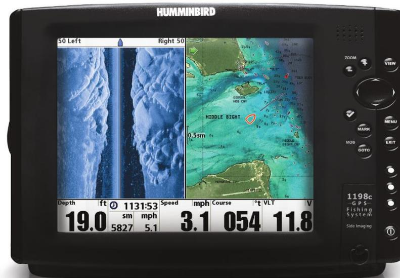
**Figure 10.** Humminbird control head view example. Left screen - Side Imaging view. Right screen - Chart view.
