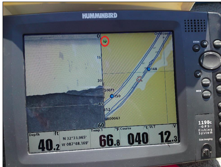
Figure 13. Example of screen with green arrow pointing to the currently “active side” (referenced by the red circle)
