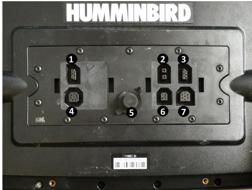
Figure 6. Rear view of the Humminbird control head with connector details. 1) Video-Out (RS-232), 2) Power, 3) GPS/Communications, 4) Video Out, 5) Ethernet, 6) Temperature/speed, and 7) Transducer
