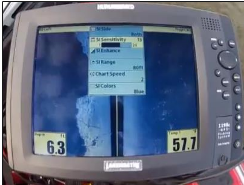
Figure 12. Sonar Menu Tab. Verify and alter these tabs accordingly to the text
