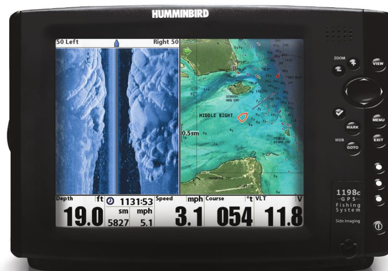
Figure 9. Humminbird control head view example. Left screen - Side Imaging view. Right screen - Chart view.
