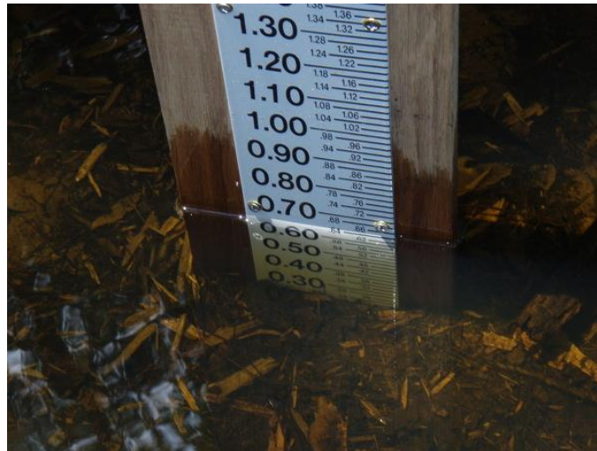
Figure 10. Example of a staff gauge. If conditions are wavy, note the mean height.
