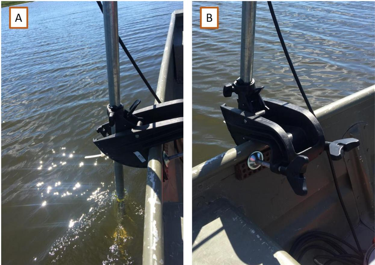
**Figure 4.** Example of pipe and trolling motor mount with transducer submerged (panel A). Shims used to make the mount more stable can be seen in panel B. The cable is fed out through the top of the pipe to be connected to the Biosonics case that contains the GPS receiver and power supply.
