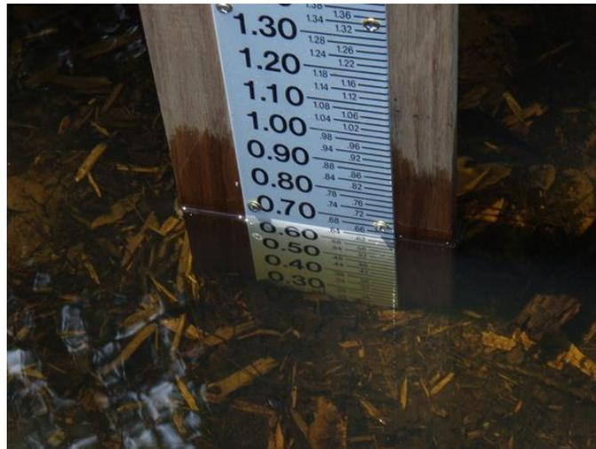
**Figure 9.** Example of a staff gauge. If conditions are wavy, note the mean height.
