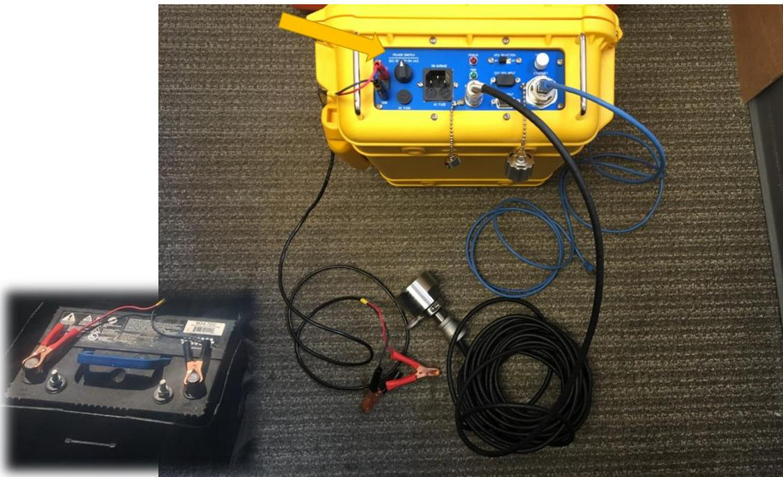
**Figure 6.** Example photo of all cables plugged into the case. Arrow points at the power switch that should be turned off until you're ready to collect data. Alligator clips should be connected to a 12V DC deep cycle battery. The sonar unit should be installed on the boat mount prior to connecting to the case.
