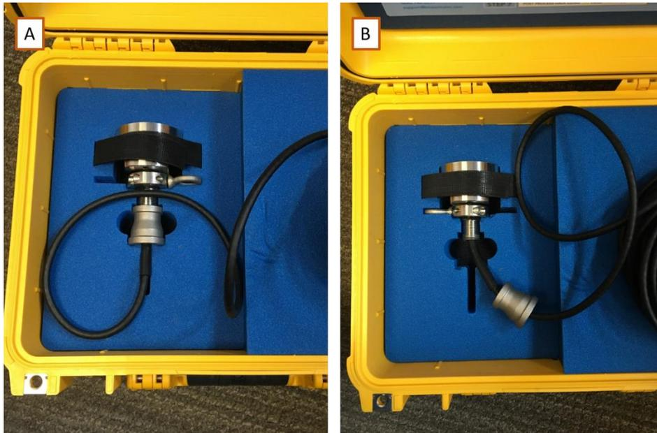
**Figure 2.** 0.5” to 0.75” reducer attached (panel A) and removed (panel B) to the sonar transducer.
