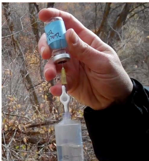
Figure 8. Transfer of dissolved gases to an evacuated gas vial.
