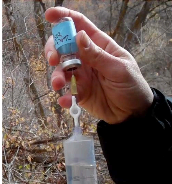
Figure 8. Transfer of dissolved gases to an evacuated gas vial
