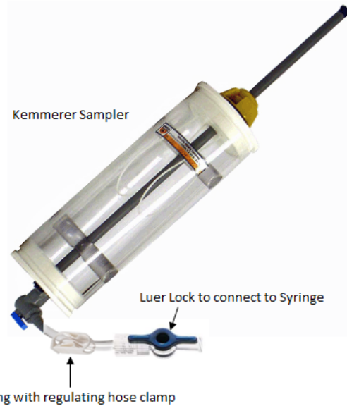
Figure 5. Tubing attachment with hose clamp and Luer-Lock to Kemmerer spigot
