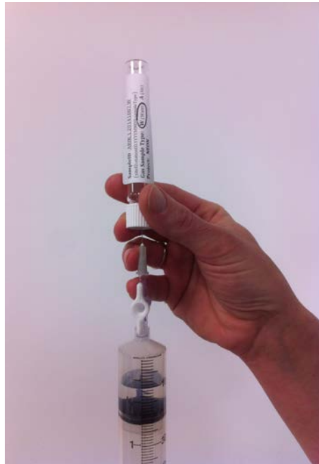
Figure 9. Transfer of dissolved gases to an evacuated gas vial.
