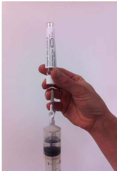
Figure 9. Transfer of dissolved gases to an evacuated gas vial.
