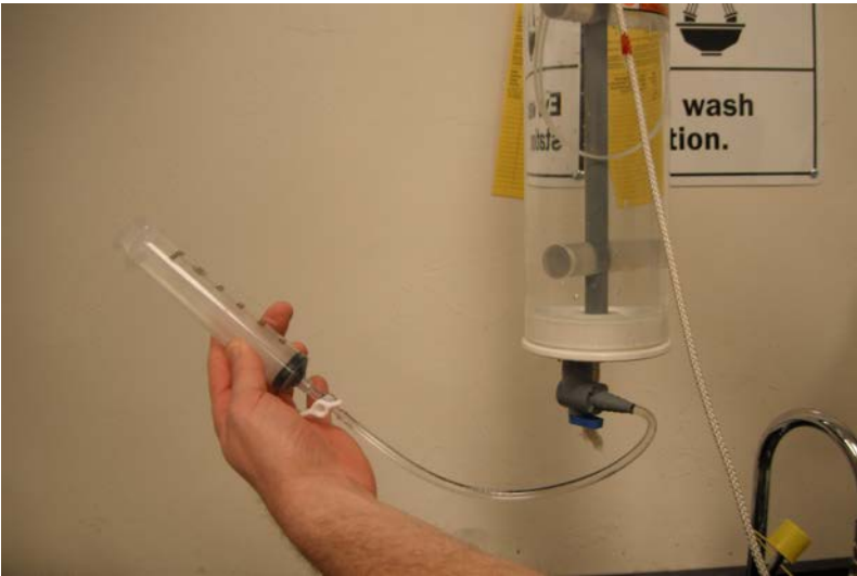
Figure 6. Syringe and 2-way stopcock attached to Kemmerer spigot
