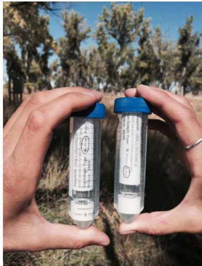
Figure 11. Dissolved gas samples stored in centrifuge tubes.
