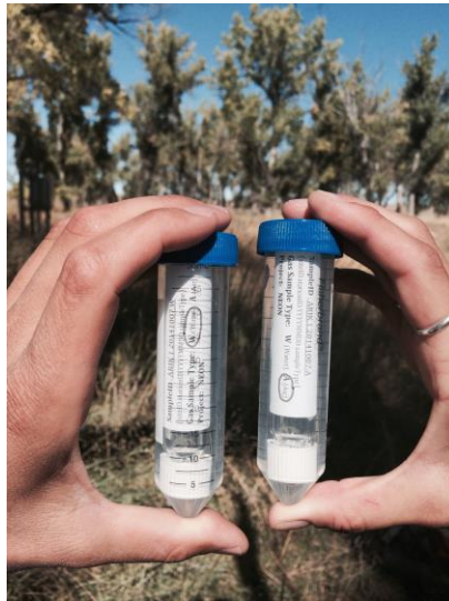
Figure 11. Dissolved gas samples stored upside-down in centrifuge tubes.
