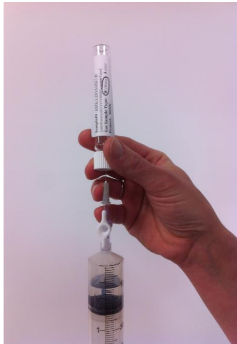
Figure 10. Transfer of dissolved gases to an evacuated gas vial.
