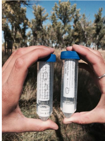
Figure 12. Dissolved gas samples stored upside-down in centrifuge tubes.
