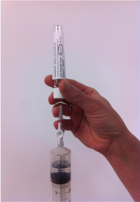
Figure 11. Transfer of dissolved gases to an evacuated gas vial.
