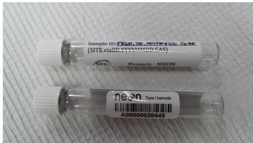
Figure 4. Example of appropriate attachment of dissolved gas vial labels. Do not tap over barcode
