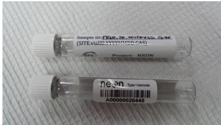
Figure 7. Example of appropriate attachment of dissolved gas vial labels. Do note tape over barcode
