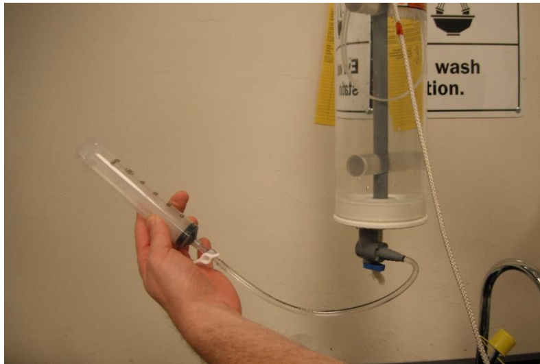
Figure 13. Syringe and 2-way stopcock attached to Kemmerer spigot
