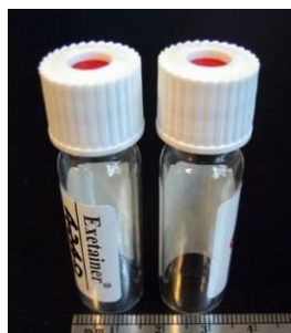
Figure 5. Gas vial with septum lid. Image from http://isotopes.forestry.ubc.ca
