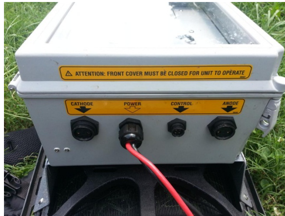
Figure 4. Cathode and anode connections on backpack electrofishing unit
