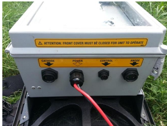
Figure 5. Cathode and anode connections on backpack electrofishing unit
