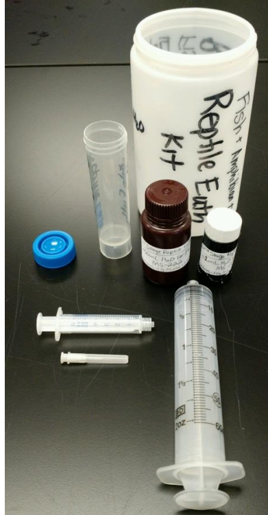
Figure 13. Reptile Euthanasia kit with 50 mL centrifuge tube to store the 5 mL syringe and needle, 60 mL HDPE amber bottle is for 1st stage solution, 20 mL HDPE scintillation vial for 2nd stage solution.
