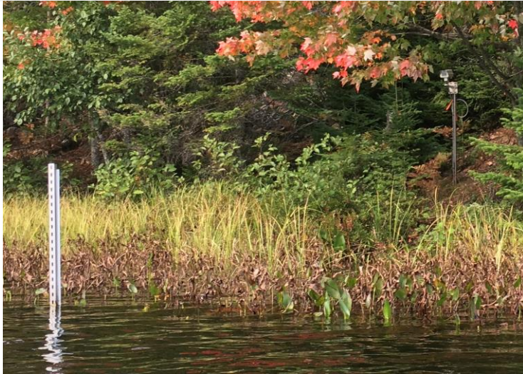
Figure 7. AIS Infrastructure: Lake Staff Gauge & Camera (Domain 05, CRAM)
