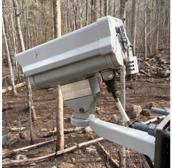
Figure 4. TIS Tower Snow Depth Camera (Domain 07, GRSM)
