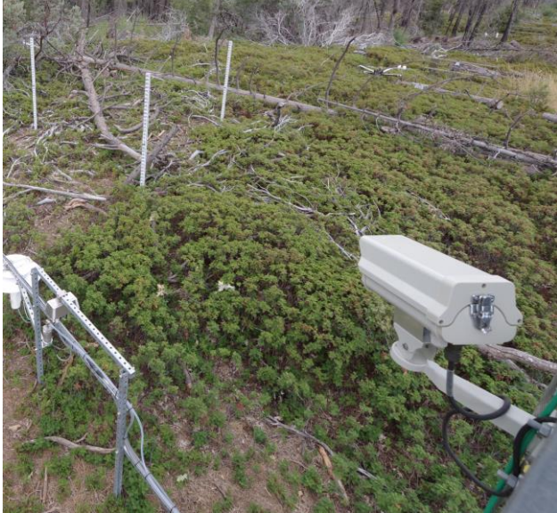
Figure 3. TIS Snow Depth Camera & Staff Gauges (Domain 17, SOAP)
