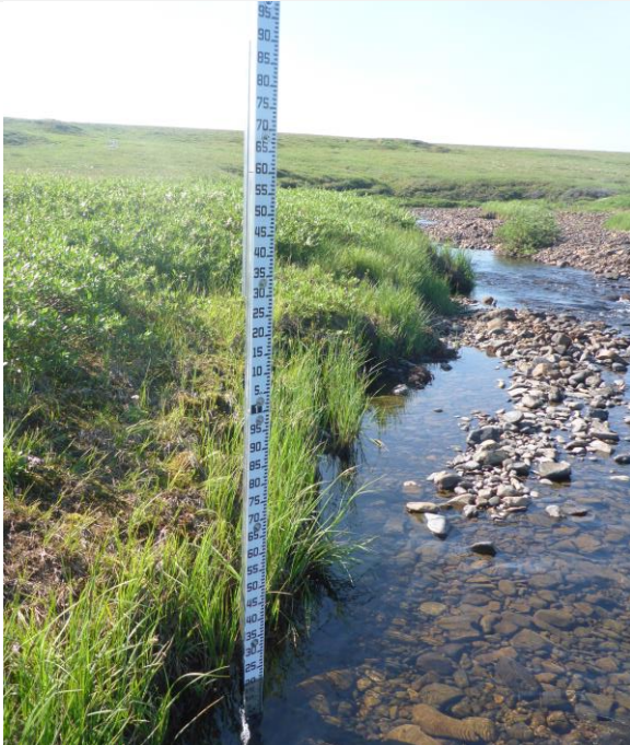
Figure 5. AIS Infrastructure: Instream Staff Gauge (Domain 18, OKSR)
