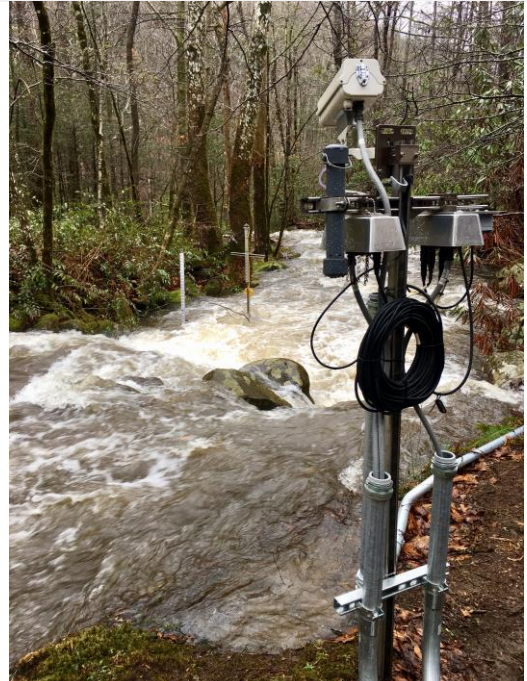
Figure 6. AIS Aquatic Stream Camera (Domain 07, LECO)
