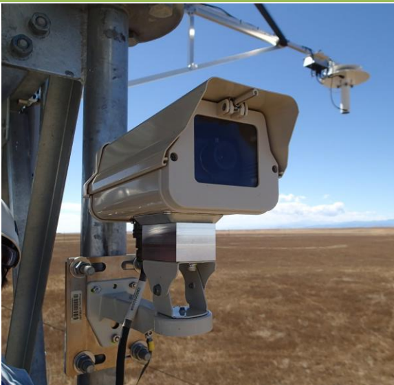
Figure 1. TIS Tower Above Canopy Camera (Domain 10, CPER)
