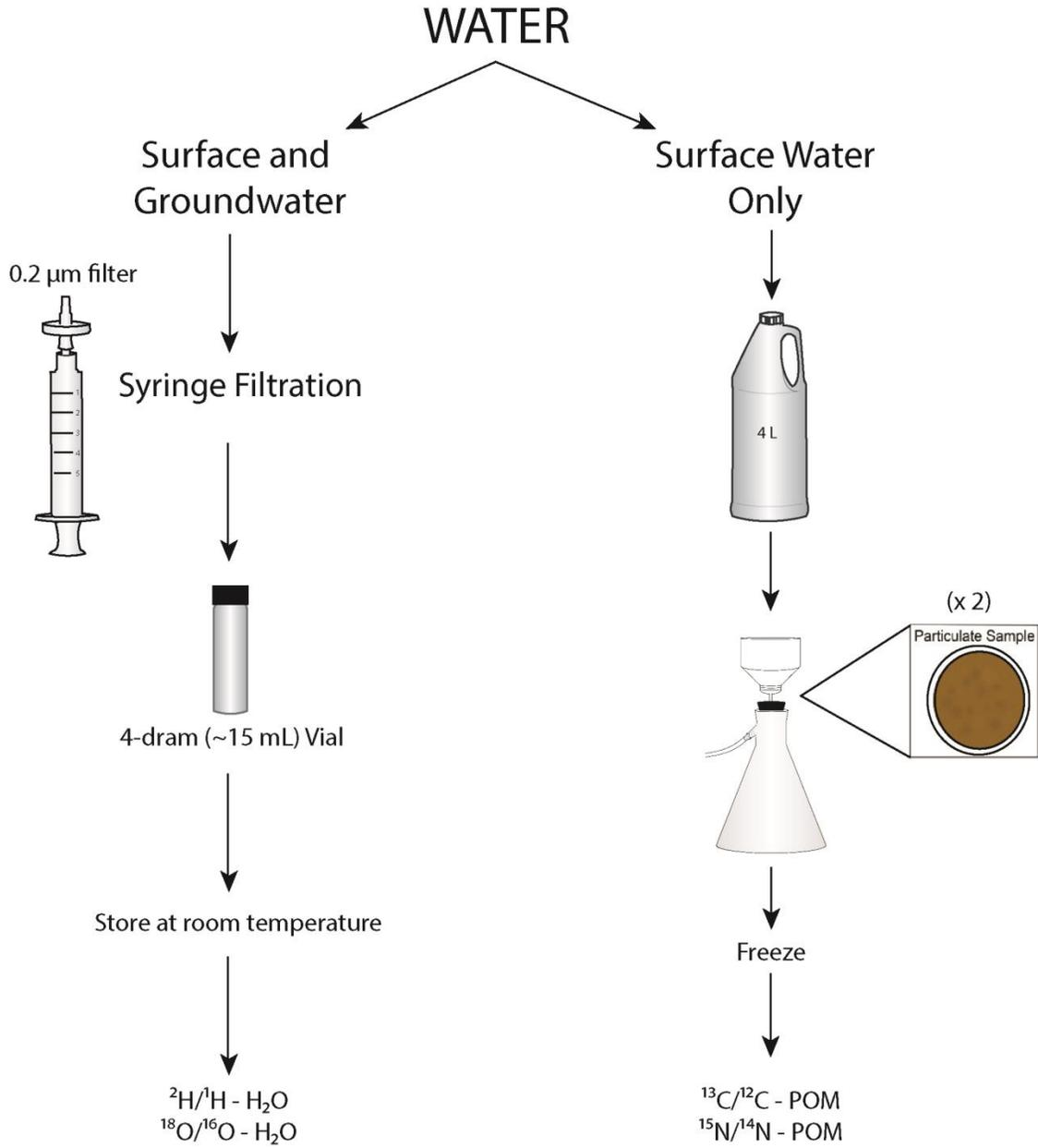
**Figure 2.** Diagram of isotope sample collection and equipment. 2 filters are collected at each collection event.
