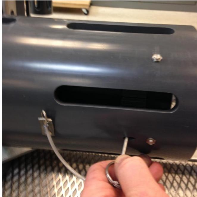
Figure 26. Remove the four locking pins
