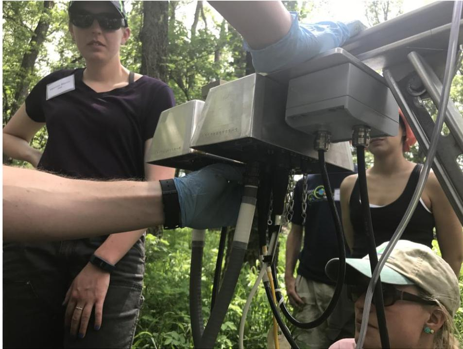
**Figure 9. Photo showing the connection of the cable assembly to the Grape for powering the sensor.**
