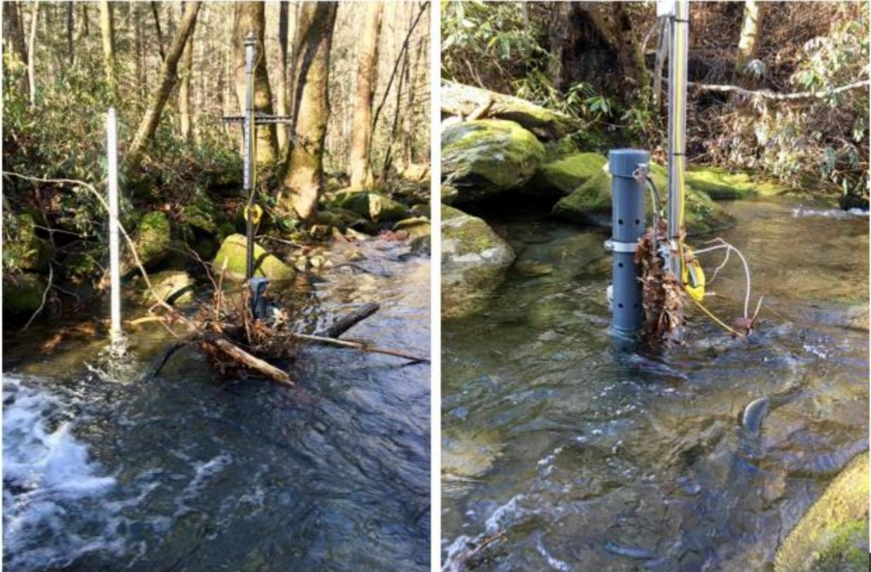
**Figure 4. Pictures of debris accumulating on sensor station after high flow event**
