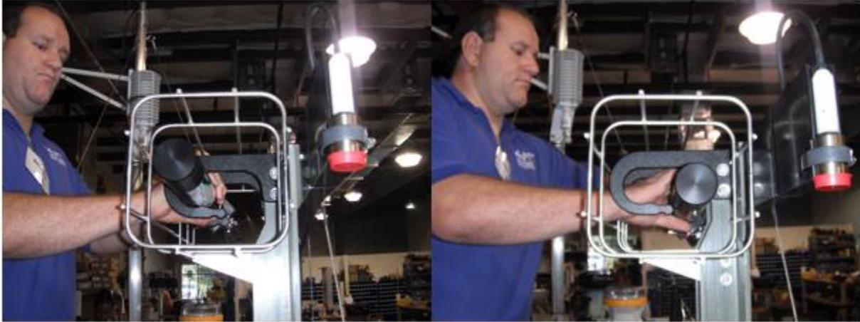
Figure 32. Removing the SUNA from the buoy deployment structure
