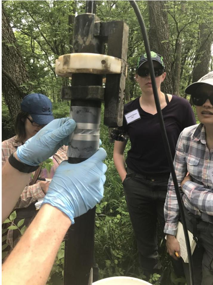
**Figure 13. Photo of Parafilm placed over optical area on SUNA nitrate analyzer**
