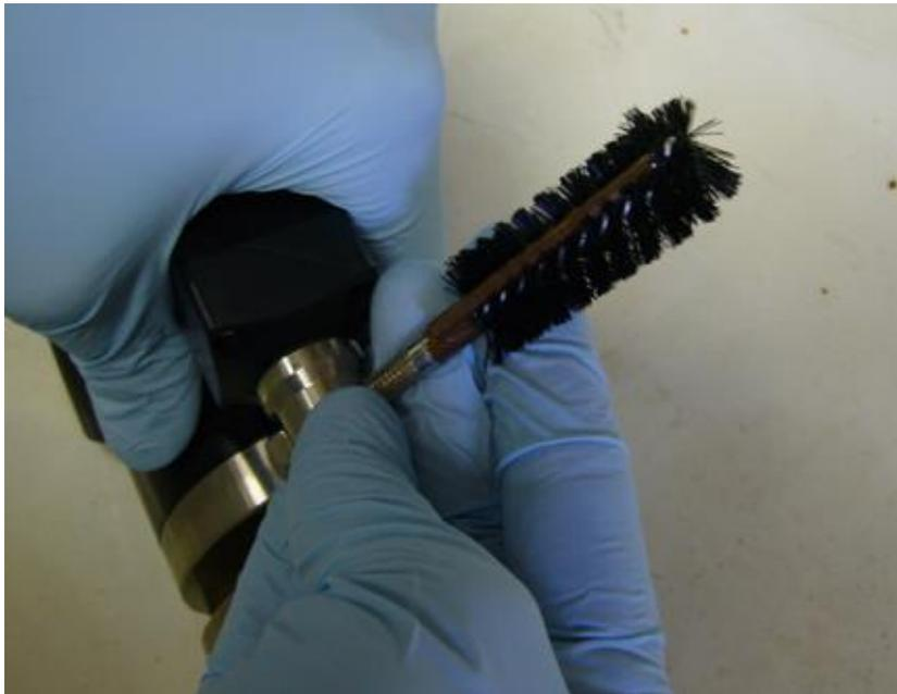
**Figure 12.** Picture of wiper being moved clear of the optical bench
