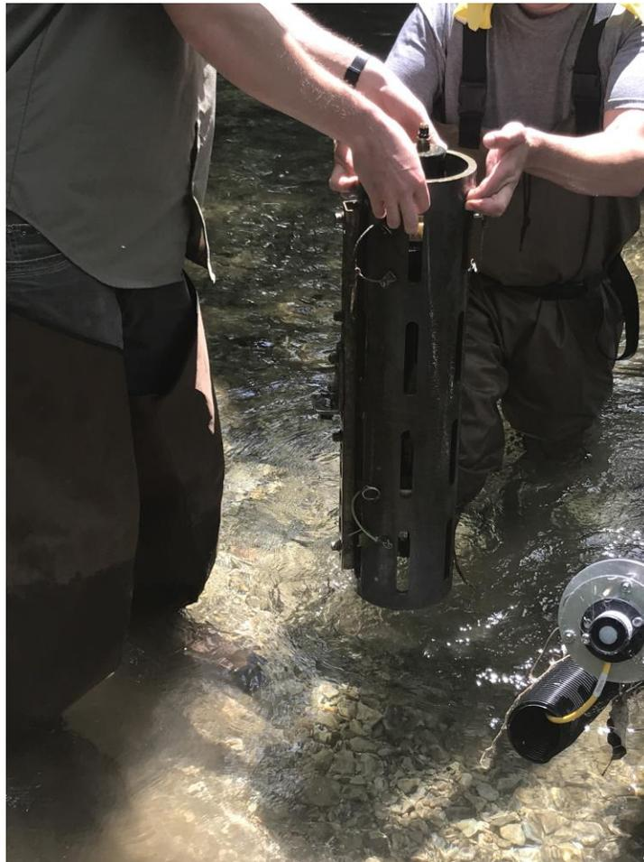
Figure 25. Photo of SUNA enclosure removal from the stream.
