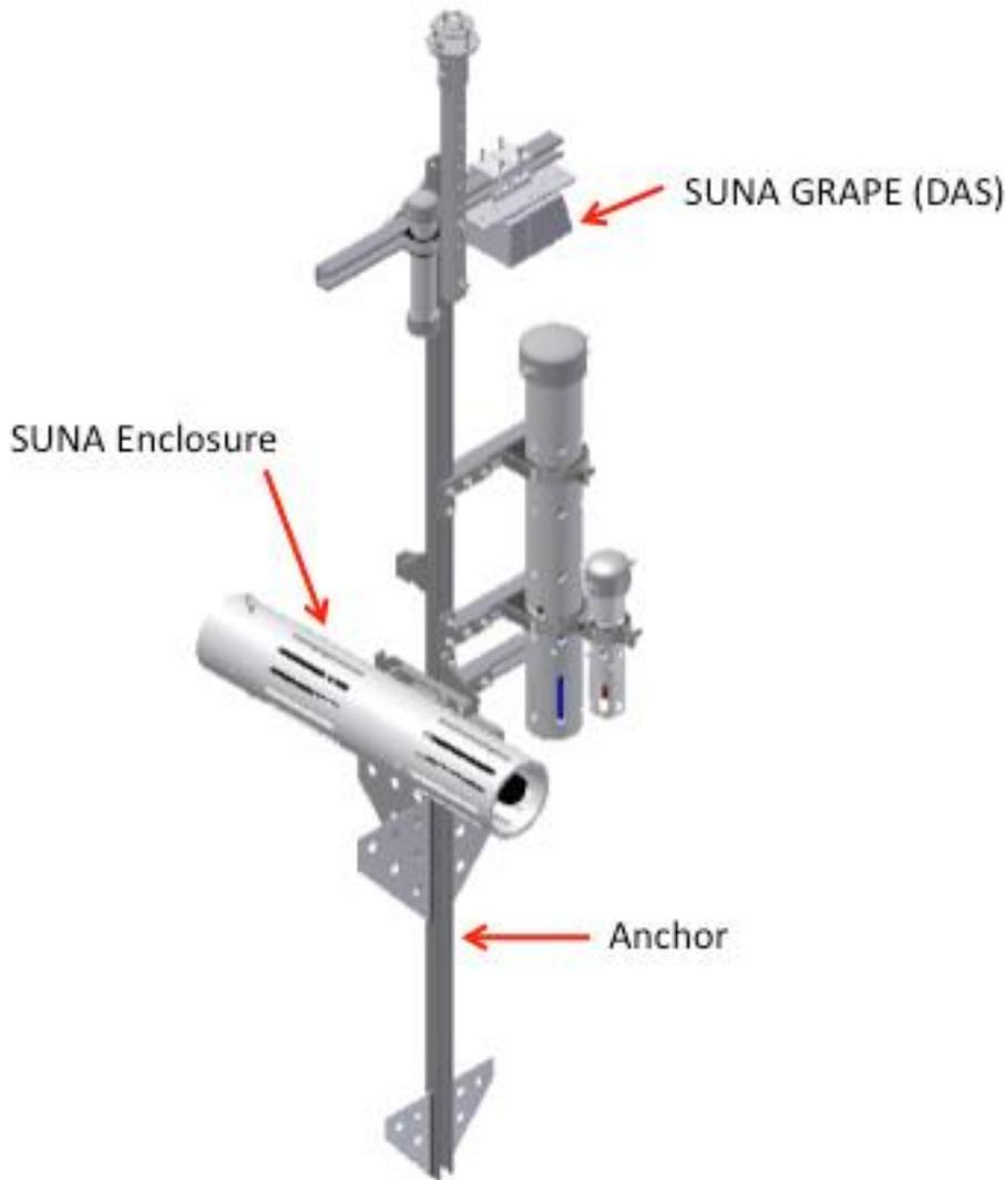
Figure 2. Schematic of infrastructure showing the location of the SUNA enclosure and Grape relative to the anchor.
