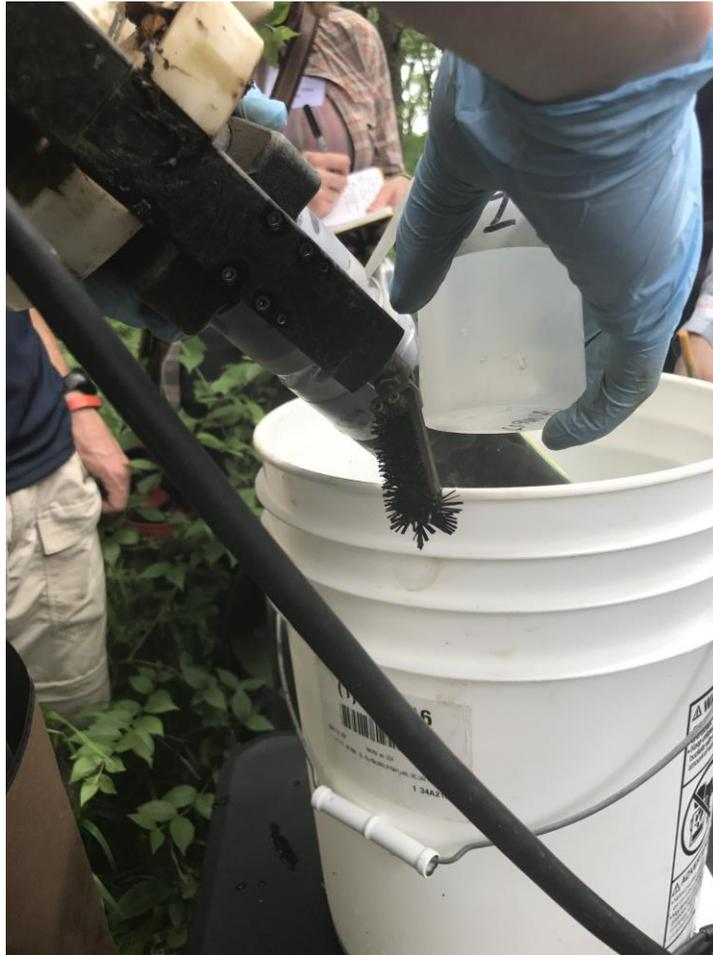
Figure 14. Photo of inserting nozzle of wash bottle to fill the optical bench with DI water
