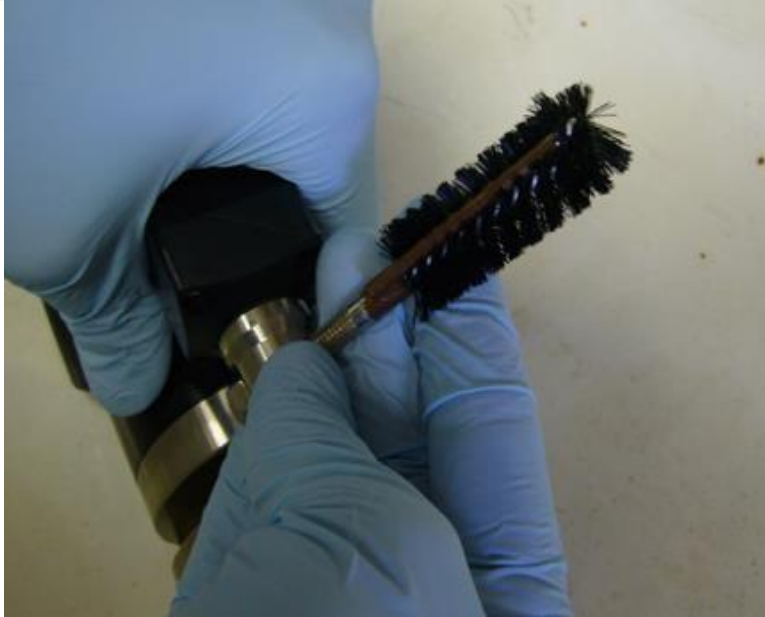
Figure 31. Physically Move Wiper on SUNA
