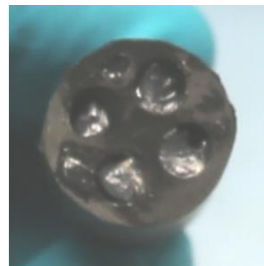
Lubricant pushed into the sockets of the connector
