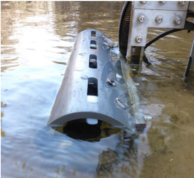
Figure 65. SUNA Partially Submerged in Stream
