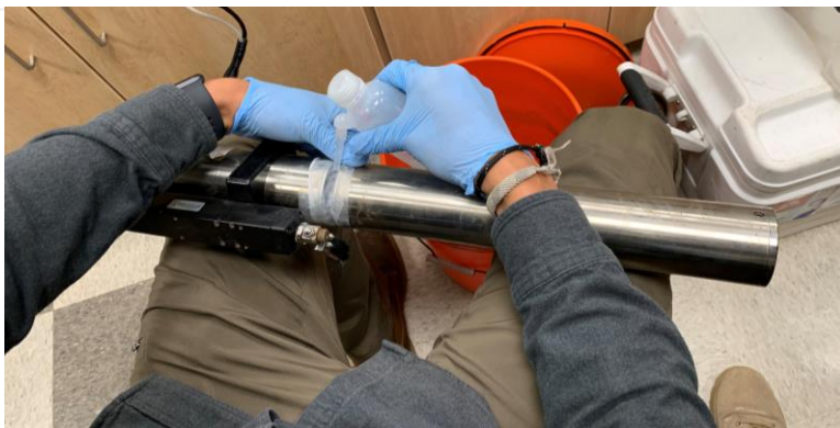
Figure 34. Fill Optical Area with Equilibrated DI Water
