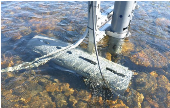
Figure 76. S2 SUNA Enclosure at D18 OKSR
