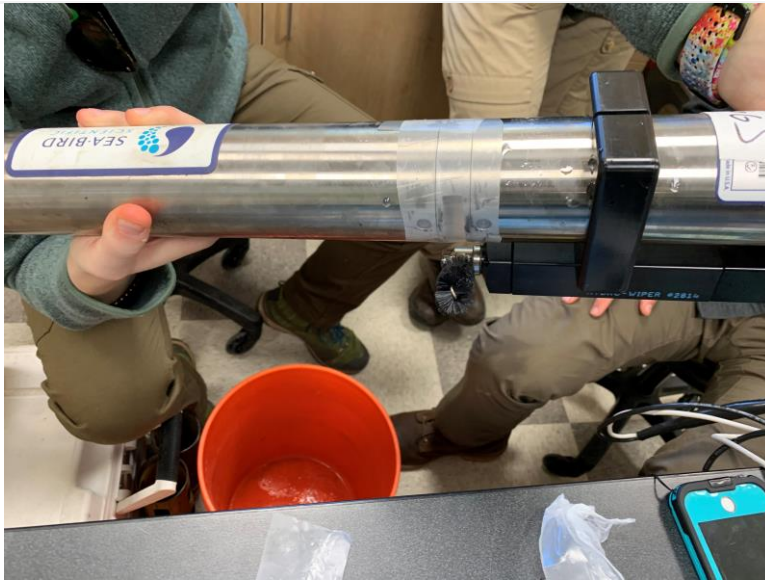
Figure 33. Wrap Parafilm around Optical Area of SUNA
