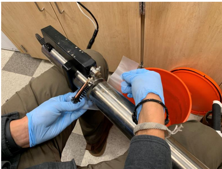
Figure 32. Cut Parafilm to Size
