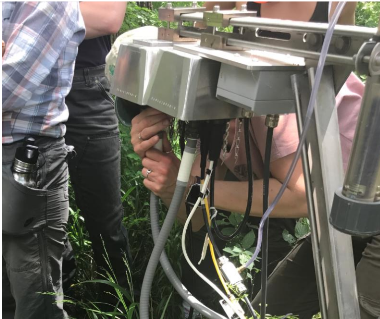
Figure 14. Disconnect the SUNA 12V Merlot Grape
