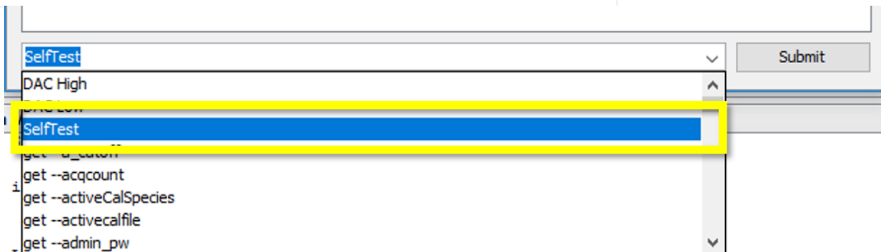
Figure 53. Select "SelfTest" in the Terminal Window
