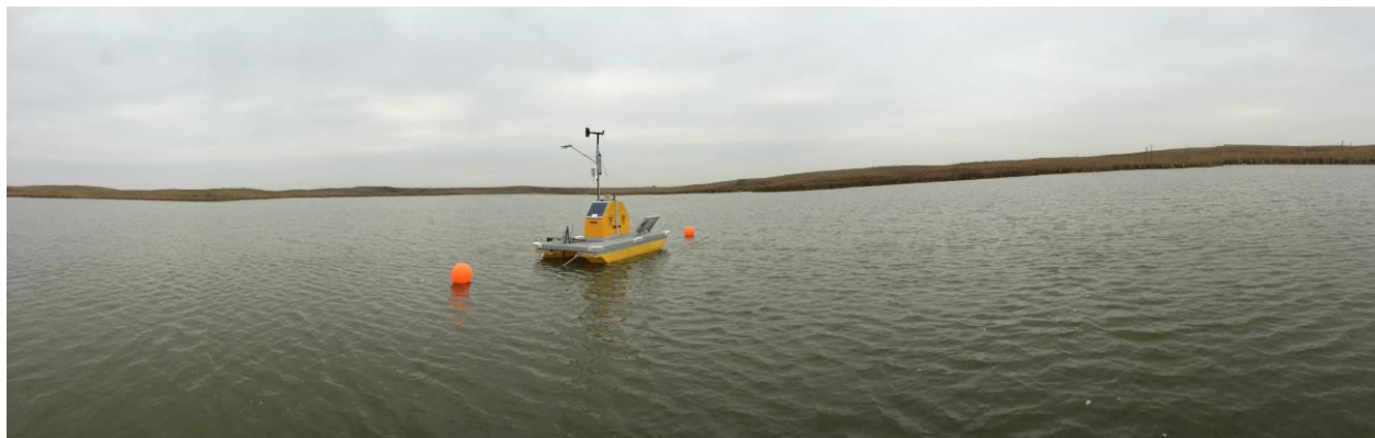
Figure 5. AIS Buoy for Lake and River Sites.
