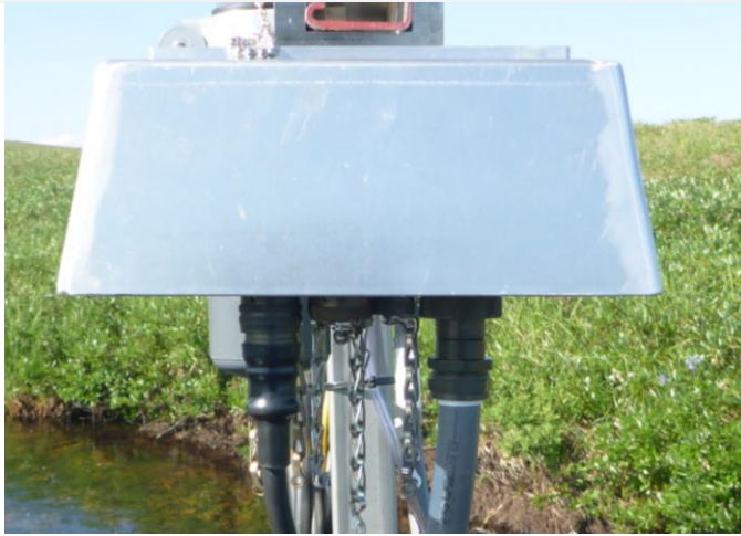
Figure 77. Reconnect Sensor Cable and Ethernet Cable to Grape
