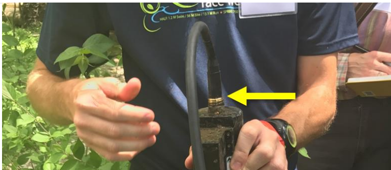
Figure 19. Connect the SUNA to the Y Cable
