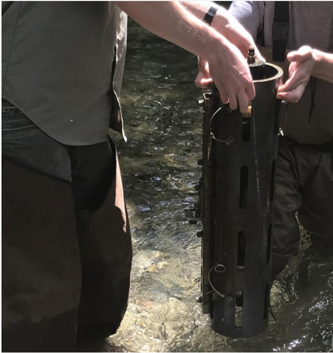
Figure 72. Remove SUNA PVC Enclosure
