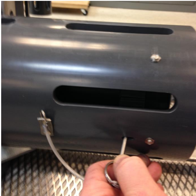
Figure 74. Pull 4 Lock Pins to Remove Captive Discs
