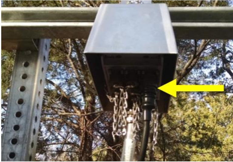
Figure 21. Attach Y-Cable to the Merlot Grape at Stream Sites
