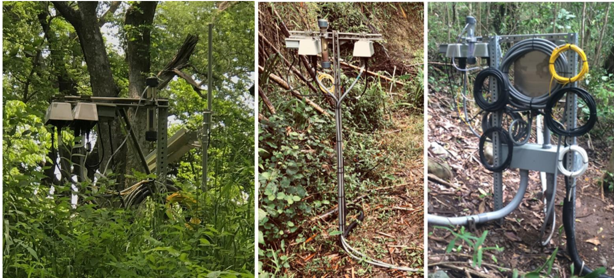
Figure 4. Stream Stand-Alone Arbors (left, middle) and Device Post Arbor (far right) .
