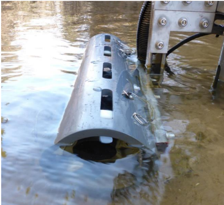
Figure 17. SUNA Mount and Enclosure in Stream Locations
