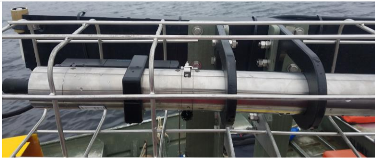
Figure 18. SUNA in Cage on Dual PAR SUNA Mount on the Buoy
