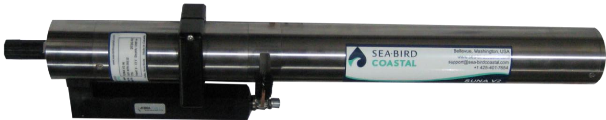
Figure 1. Sea-Bird Scientific SUNA V2 with Integrated Anti-Fouling Wiper.
