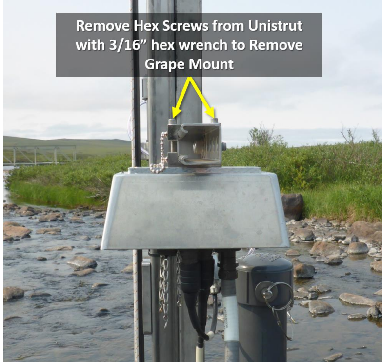
Figure 11. Remove Grape Shield with 3/16" Hex Wrench
