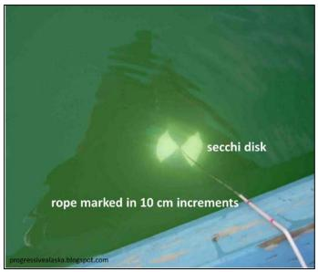
Figure 3. Example of a Secchi disc underwater.
