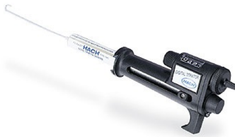
Figure 17. Digital titrator with titrant cartridge and titration tube attached. Photo from the Hach Digital titrator manual.
