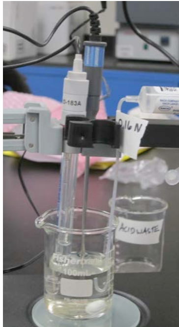
Figure 19. Diagram of titration set-up with digital titrator, stir bar, pH meter and temperature probe. Ensure nothing is touching the sides and bottom of the beaker or the stir bar
