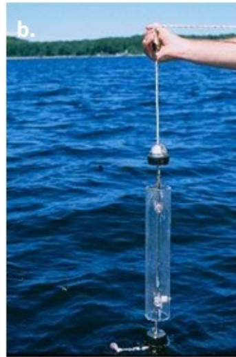
Figure 9. Illustration of Kemmerer sampler for water sampling (a). Illustration of how the Kemmerer is lowered into the water by holding the rope and messenger (b)
