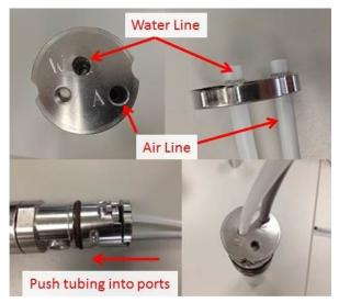
Figure 14. Attaching grey air-line and white water-lines to pump
