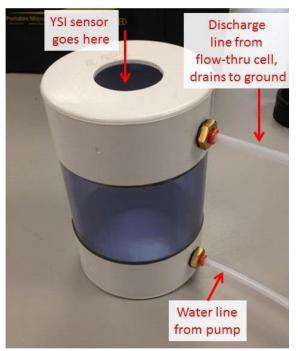
Figure 18. White water-line to flow-thru cell.
