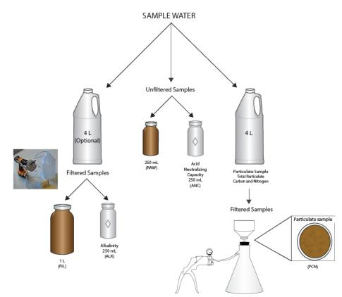
Indicates sample bottles that will remain at the Domain Support Facility for analysis. Letters in parenthesis indicate the codes that correspond to the chemistry labels.
