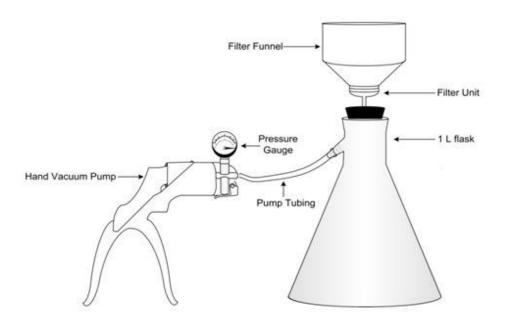
**Figure 21.** Filter apparatus set-up for particulates, using a) the vacuum pump and filter manifold, and b) the hand vacuum pump attached to the filter flask and filter funnel.
