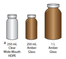
**Figure 4.** Water chemistry bottle types. <sup>a</sup> indicates sample bottles that will remain at NEON Domain Support Facilities to be analyzed. These bottles are labeled with different labels (Figure 6) and bottles can be re-used. 125 mL bottles may be used if less volume is needed – site specific.
