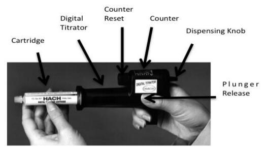
Figure 22. Inserting titrant cartridge into digital titrator. Photo from the Hach Digital titrator manual
