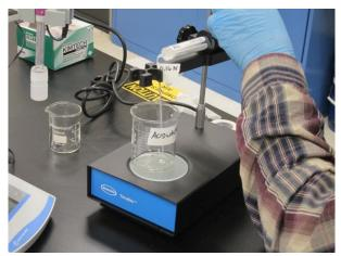
**Figure 24.** Diagram of procedure to expel acid from digital titrator set-up into a temporary acid waste container.
