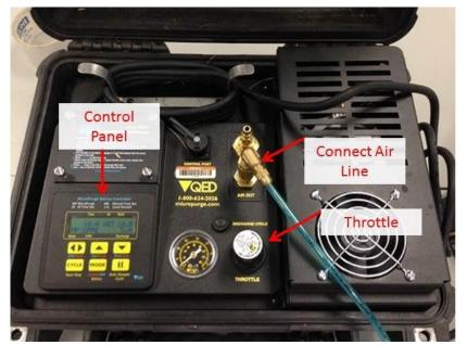
Figure 16. Attach blue air-line to controller
