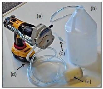
**Figure 20.** Pump and filter setup, including (a) a peristaltic sampling pump (modified from Woessner 2007), (b) a 4 L sample bottle, (c and d) tubing connectors to connect peristaltic and C-flex tubing, and (e) a capsule filter
