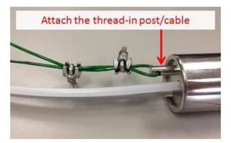
Figure 15. Attach post and cable to the pump
