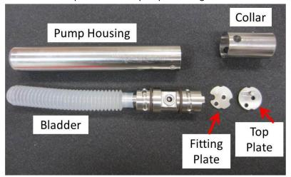
Figure 13. Components of the sampling pump
