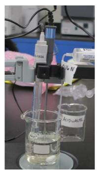
**Figure 25.** Image of titration set-up with digital titrator, stir bar, pH meter and temperature probe. Ensure nothing is touching the sides and bottom of the beaker or the stir bar
