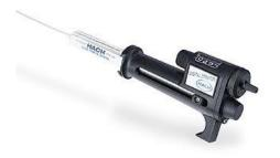
**Figure 23.** Digital titrator with titrant cartridge and titration tube attached. Photo from the Hach Digital titrator manual.
