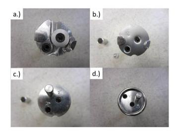
**Figure 12**. Assembly of the fitting plate at the top of the pump for holding the air and water lines. (a) Bare top of pump. (b) Fitting plate added ("TOP" must face upwards). (c) Top plate added. (d) Collar added to lock parts (a-c) together.
