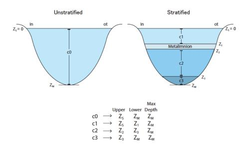
**Figure 9.** Example of an unstratified and stratified lake water column a) sampling depths with placement of thermocline and b) identification of upper and lower section depths. In deep lakes, 2 thermal stratifications may occur, creating 3 sections.
