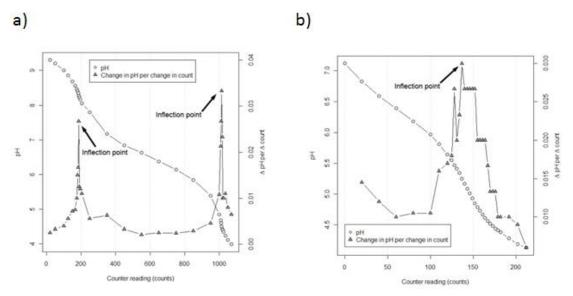
**Figure 26.** Example of inflection point titration using a digital titrator of a) a high alkalinity sample and b) a low alkalinity sample. Note difference in Y-axis scale. (Modified from USGS TWRI Book 9, Alkalinity, Version 3.0 7/2006).
