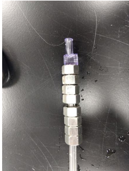
Figure 22. Nuts added to peristaltic pump tubing for weight.
