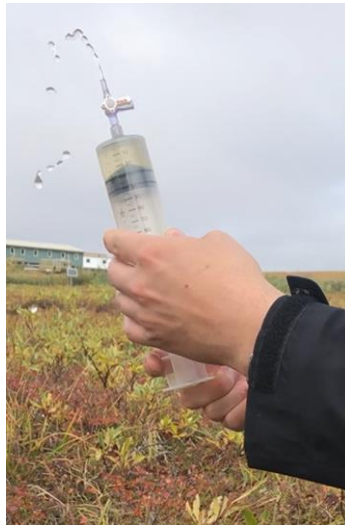
Figure 25. Expel air bubbles from the syringe during bubble-free sampling.
