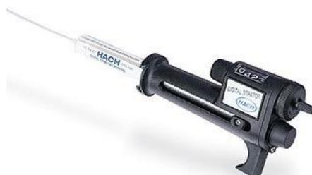
**Figure 25.** Digital titrator with titrant cartridge and titration tube attached. Photo from the Hach Digital titrator manual.
