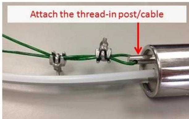
**Figure 16.** Attach post and cable to the pump via the top plate
