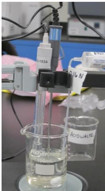
**Figure 27.** Image of titration set-up with digital titrator, stir bar, pH meter and temperature probe. Ensure nothing is touching the sides and bottom of the beaker or the stir bar
