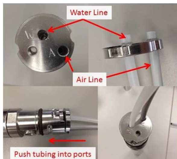
Figure 15. Attaching grey air-line and white water-lines to pump (top-right photo shows lines pushed through top plate and “teeth” of grab plate)
