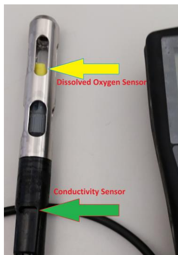
Figure 6. Picture of handheld meter showing location of sensors on probe.
