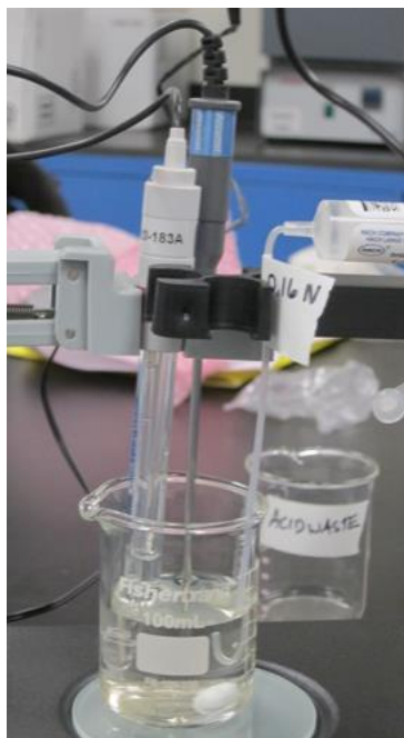
Figure 30. Image of titration set-up with digital titrator, stir bar, pH meter and temperature probe. Ensure nothing is touching the sides and bottom of the beaker or the stir bar
