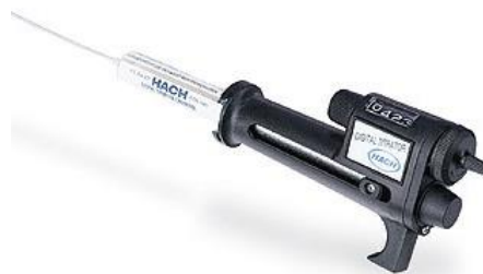
Figure 24. Digital titrator with titrant cartridge and titration tube attached. Photo from the Hach Digital titrator manual.
