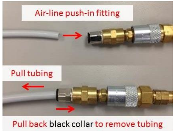
Figure 18. Attach grey air-line to blue air-line
