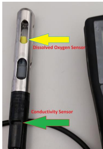
Figure 7. Picture of handheld meter showing location of sensors on probe.
