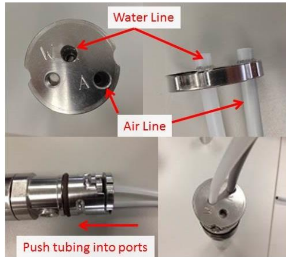
Figure 15. Attaching grey air-line and white water-lines to pump
