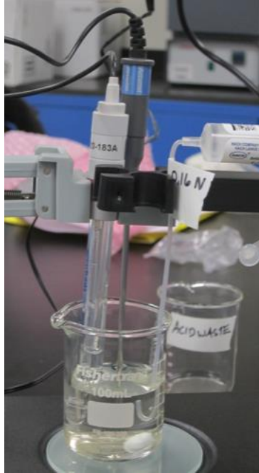
Figure 26. Image of titration set-up with digital titrator, stir bar, pH meter and temperature probe. Ensure nothing is touching the sides and bottom of the beaker or the stir bar
