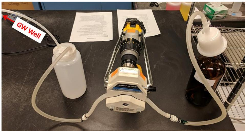
**Figure 31.** Filtering setup to minimize sample aeration during filtration for low-flow and minimum purge groundwater samples.
