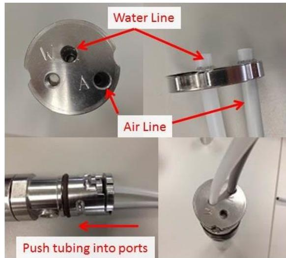
**Figure 19.** Attaching grey air-line and white water-lines to pump (top-right photo shows lines pushed through top plate and “teeth” of grab plate)
