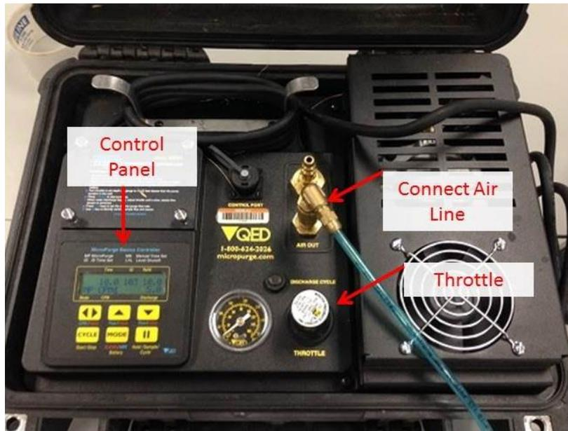
**Figure 21.** Attach blue air-line to controller.
