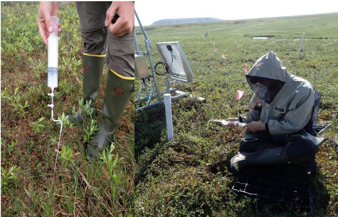
**Figure 28.** Sampling needle and syringe setup.
