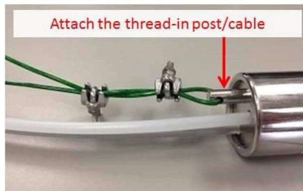
**Figure 20.** Attach post and cable to the pump via the top plate.
