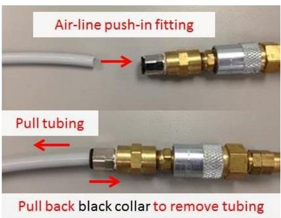
Figure 22. Attach grey air-line to blue air-line.
