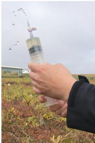
**Figure 29.** Expel air bubbles from the syringe during bubble-free sampling.
