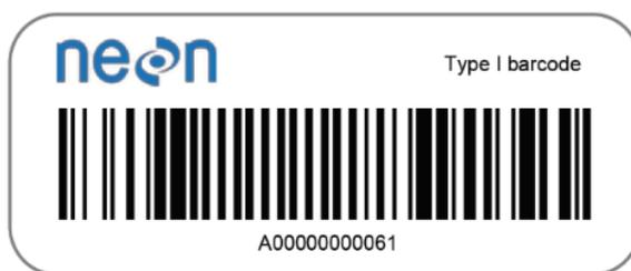
**Figure 7.** An example of a Type I barcode. These large-size, field-tolerant barcodes have a prefix of 'A' followed by 11 numbers.
