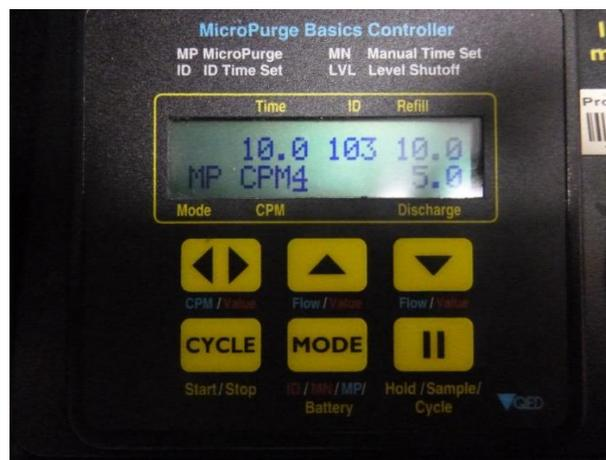
**Figure 24.** Groundwater pump control panel screen. Note the Refill and Discharge times on the right.
