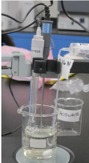
**Figure 39.** Image of titration set-up with digital titrator, stir bar, pH meter and temperature probe. Ensure nothing is touching the sides and bottom of the beaker or the stir bar
